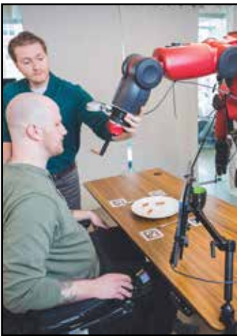
Cleveland State University engineering students test an assistive robotic feeding device.
