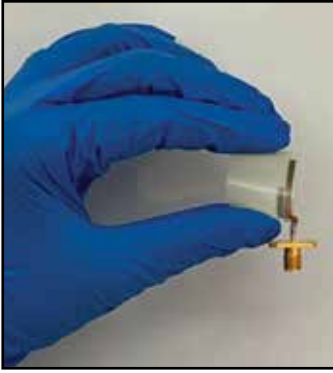
Youngstown State University's microstrip antenna is printed on a flexible substrate.
