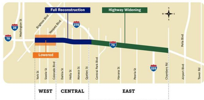
The I-70 project has three main components. The flooding happened in the lowered portion. Retrieved from Colorado DOT.
