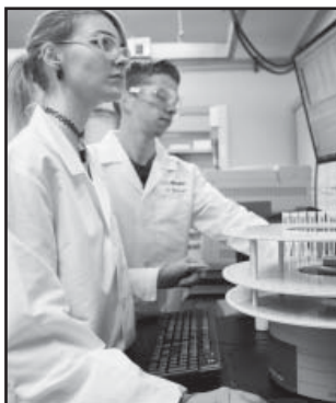
OU chemical engineering juniors, Mira Cooper & Joshua Greenlee, use an ion chromatograph to study how scale forms within industrial boilers.
